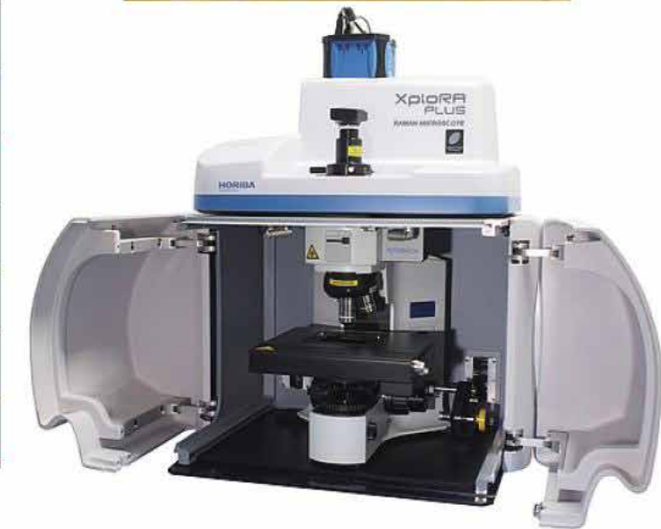
Figure 3: (Left) Raman spectra recorded on different polymer families. (Top right) Aluminum strip pellet containing 12 tablets sent to participants, that were to be dissolved in analytical grade water to control background contamination. (Bottom right) HORIBA Xplora PLUS Raman microscope with class I laser enclosure used for this study.
