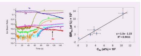
Quantification of As • Comparison with SIMS • Good agreement down to 10<sup>17</sup> atoms/cm<sup>3</sup> • Fast Control Tool (1 μm film in 60 s) PVSat 2013 Proceedings, Kartopu et al, CSER, UK.
